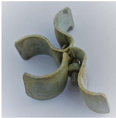
Photos show examples of unstable panels due to missing clamps and a damaged imported clamp recovered from a temporary fence in North Queensland.
